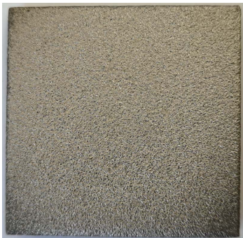
图 16 喷丸强化后试件的表面形貌 Fig.16 Surface morphology of the specimen after shot peening
