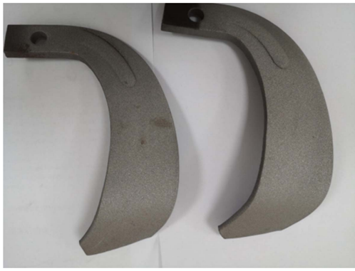
图 13 喷涂加工得到的旋耕刀样件 Fig.13 Rotary tiller blade samples processed with arc spraying
