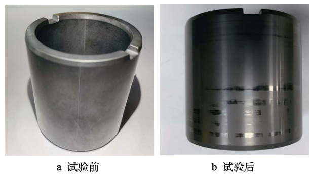
图 7 试验试件轴套展示 Fig.7 Experimental specimen sleeve display: a) before the test; b) after the test
