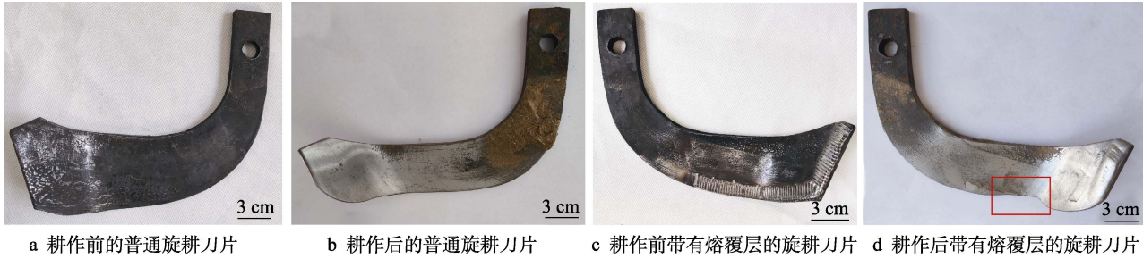
图 13 普通旋耕刀与带有熔覆层旋耕刀作业前后对比 Fig.13 Comparison of ordinary rotary blade and rotary blade with cladding layer before and after operation: a) ordinary rotary blade before cultivation; b) ordinary rotary tillage blades after cultivation; c) rotary tillage blades with a fusion layer before cultivation; d) rotary tiller blades with fusion layer after cultivation
