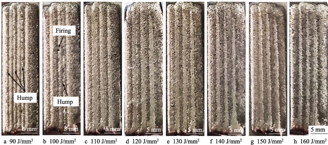
图 2 不同激光功率下镍基熔覆层的宏观形貌 Fig.2 Macromorphology of nickel base cladding layer with different laser power
