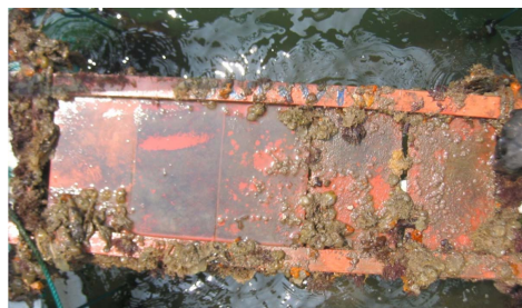
图 4 静态浅海浸泡样板 24 个月防污效果 Fig.4 Antifouling effect of sample plate after static shallow water immersion for 24 months
