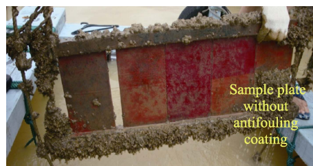
图 6 三亚静态实海浸泡样板 24 个月防污效果 Fig.6 Antifouling effect of sample plate after static sea immersion for 24 months in Sanya
