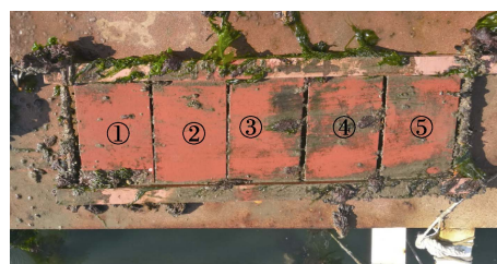
图 3 静态浅海浸泡样板 24 个月防污效果 Fig.3 Antifouling effect of sample plate after static shallow water immersion for 24 months
