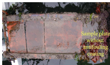
图 5 青岛静态实海浸泡样板 24 个月防污效果 Fig.5 Antifouling effect of sample plate after static sea immersion for 24 months in Qingdao
