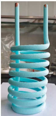
图 3 喷涂固化后的铜基换热器 Fig.3 Spray-cured copper-based heat exchanger
