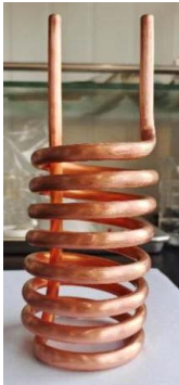
图 2 预处理后的铜基换热器 Fig.2 Pretreated copper-based heat exchanger
