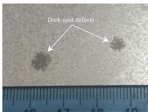
图 1 Zn-11Al-3Mg 镀层表面黑点缺陷宏观照片 Fig.1 Macro appearance of the dark spot defects on Zn-11Al-3Mg coating
