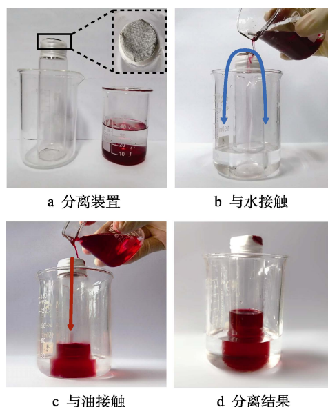
图 9 超疏水/超亲油镍网的油水分离示意图 Fig.9 Schematic diagram of oil-water separation of superhydrophobic/superoleophilic nickel mesh: a) separation device; b) contact with water; c) contact with oil; d) separation results
