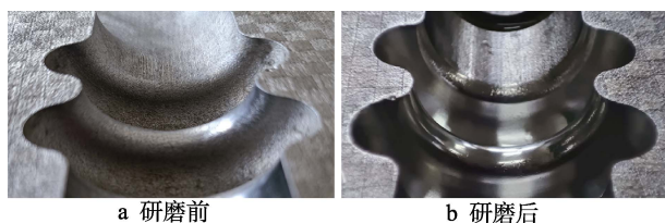
图 13 工件二维宏观形貌对比 Fig.13 Comparison of 2D macro morphology of workpiece: a) before grinding; b) after grinding
