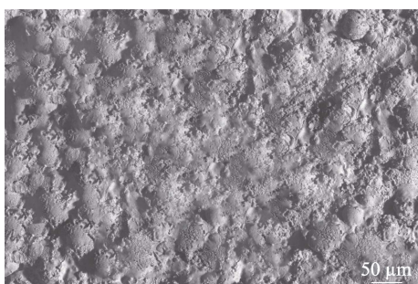
图4 Ni60涂层的表面形貌 Fig.4 Surface morphology of Ni60 coating
