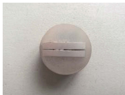
图7 经冷镶嵌后的镁合金截面试样 Fig.7 Cross-sectional specimen of magnesium alloy after cold inlay
