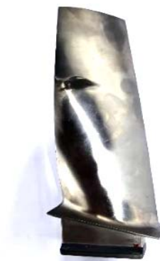
图 2 某型 TC4 钛合金叶片 Fig.2 TC4 titanium alloy blade of certain aero-engine
