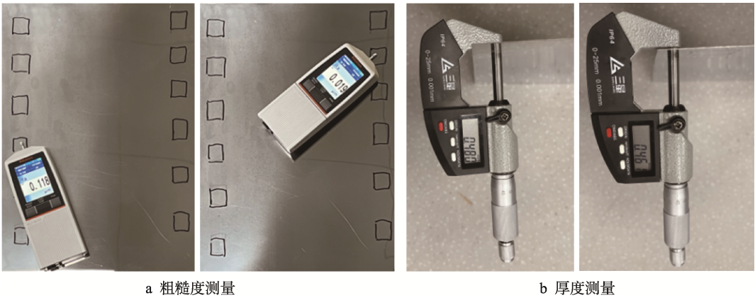
图 11 工件抛光前后粗糙度和工件厚度的测量 Fig.11 Measurement of roughness value and workpiece thickness before and after polishing: a) roughness measurement; b) thickness measurement
