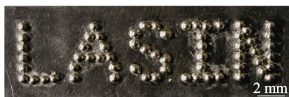
图8 二维金属液滴沉积 [48] Fig.8 2D metal droplet deposition [48]
