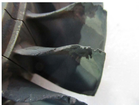
图 10 进场分解后发现的涡轮叶尖损伤情况 Fig.10 Damage to turbine blade tip found after approach and decomposition
