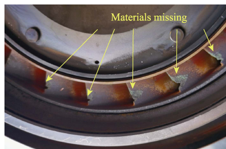
图 6 涡轮导向叶片后缘材料缺失 Fig.6 Missing material on the trailing edge of turbine guide vanes
