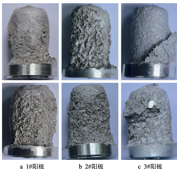
图 8 清洗腐蚀产物后的阳极表面形貌 Fig.8 The surface morphologies of the anodes after cleaning the corrosion products: a) 1# anode; b) 2# anode; c) 3# anode
