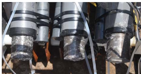
图1 深海环境下 FTR 试验用阳极表面照片 Fig.1 Surface photo of anodes for FTR test in deepwater environment
