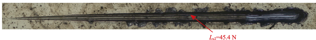
图 5 多层 TiN/Ti 涂层的划痕形貌 Fig.5 Scratch morphology of TiN/Ti multilayer coating
