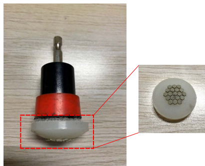
图6 固结磨料小工具头 Fig.6 Fixed abrasive tool head
