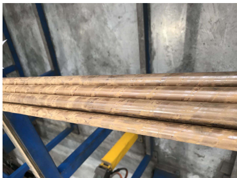
图 1 表面带氧化皮缺陷的钛合金棒材 Fig.1 Titanium alloy bar with oxide skin defect
