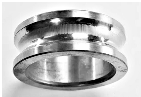
图2 产生电蚀损伤后的轴承滚道面面貌 Fig.2 Morphology of the bearing raceway after electrical corrosion
