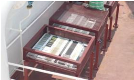
图 3 远洋船舶移动平台样品投试情况 Fig.3 Photo of sample putting on ocean-going ship platform
