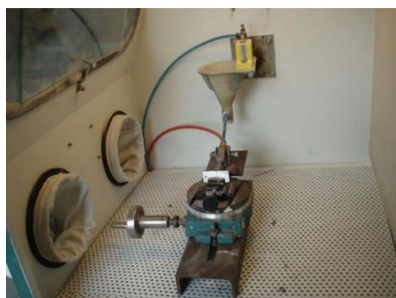
图13 粒子冲刷试验机 [59] Fig.13 Particle erosion test machine [59]
