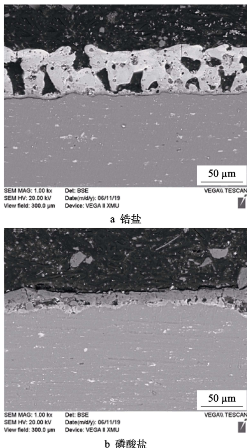
图2 微弧氧化处理后截面形貌 Fig.2 Section morphology after micro-arc oxidation treatment: (a) zircon salt, (b) phosphate
