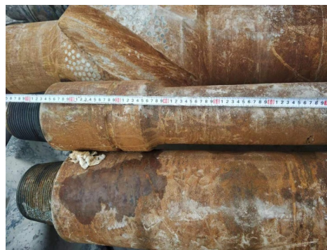
图 1 现场刺漏钻杆宏观形貌 Fig.1 Macroscopic appearance of drill pipe
