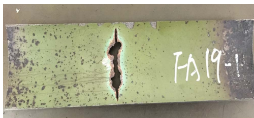
a 1#钻杆内壁涂层及刺孔形貌
