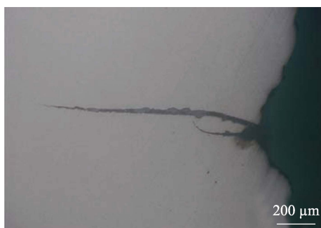
图 11 1#样品腐蚀坑底部裂纹金相形貌 Fig.11 Metallographic appearance of bottom crack of corrosion pit of sample 1#
