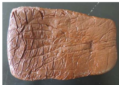
图1 所用防火泥外观 Fig.1 Appearance of fireproofing mud
