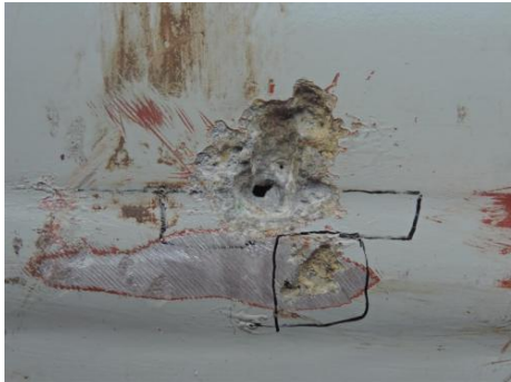
图 2 近海某变 GIS 筒体铝管腐蚀穿孔外部形貌 Fig.2 External morphology of GIS cylinder aluminum tube corroded and perforated in a main transformer in offshore
