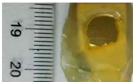
图 9 耐盐雾测试 6 个月后表面的宏观形貌 Fig.9 Surface macroscopic image of sample after neutral salt spray test for 6 months
