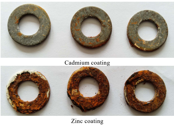
图 15 机械镀镉与机械镀锌试样的盐雾试验结果 Fig.15 Salt spray test results of mechanical cadmium plating and mechanical galvanizing
