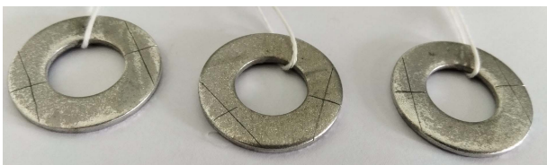
图 14 划格试样在 5% 的氯化钠溶液中浸泡 250 h Fig.14 Cross-cut sample immersed in 5% sodium chloride solution for 250 h
