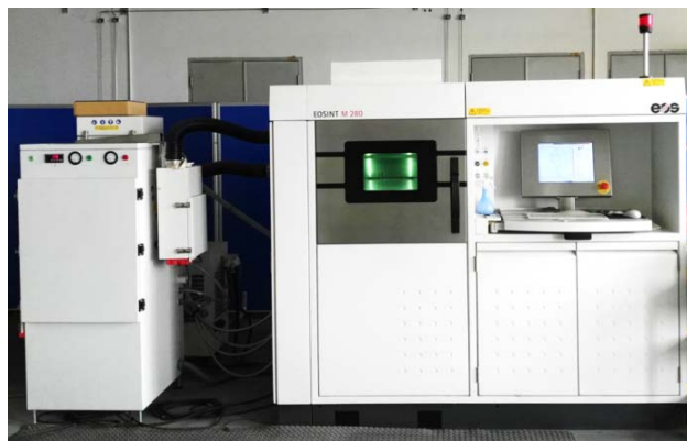
图 1 EOS INT M280 金属快速成形机 Fig.1 EOSINTM280metal rapid forming machine
