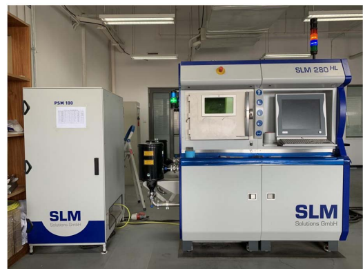
图 1 SLM Solutions M280 金属快速成形机 Fig.1 SLM Solutions M280 metal rapid prototyping machine
