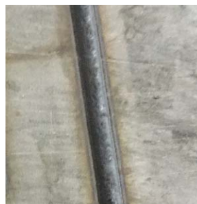
图 10 单向单道熔覆层表面形貌 Fig.10 Surface profile of single-directional cladding layer
