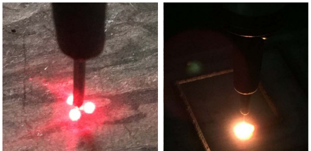
图 8 光丝耦合图 Fig.8 Coupling of beams and wire
