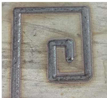
图 11 多向单道熔覆层表面形貌 Fig.11 Surface morphology of multi-directional cladding layer
