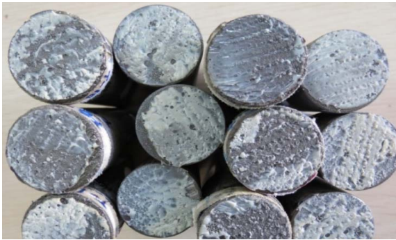
图 5 复合热源喷涂 WC-10Co4Cr 涂层拉断后外观形貌 Fig.5 Appearance of the LHPS WC-10Co4Cr coatings after the tension test
