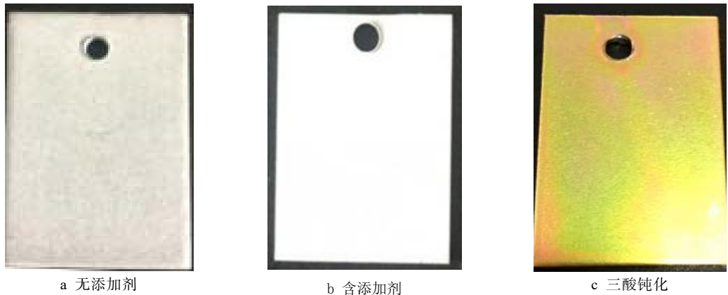
图 7 镀层外观 Fig.7 Appearance of coating: a) without additives; b) with additives; c) tri acid passivation
