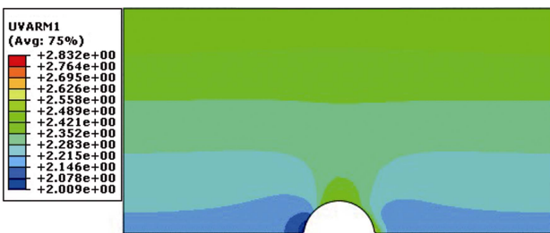
图 3 冷却热震 5 s 时 TC 层失效能密度分布云图 Fig.3 Distribution of failure energy density for TC layer during thermal shock for 5 s
