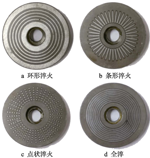
图 3 激光淬火球墨铸铁表面形貌 Fig.3 Surface morphology of laser quenching ductile iron: a) ring quenching; b) strip quenching; c) point quenching; d) full quenching
