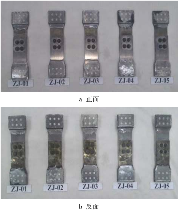
图 6 第 5 周期钢-钛搭接件宏观腐蚀形貌图 Fig.6 Macroscopic corrosion morphology of steel-titanium lap joints in the fifth cycle: a) front, b) back
