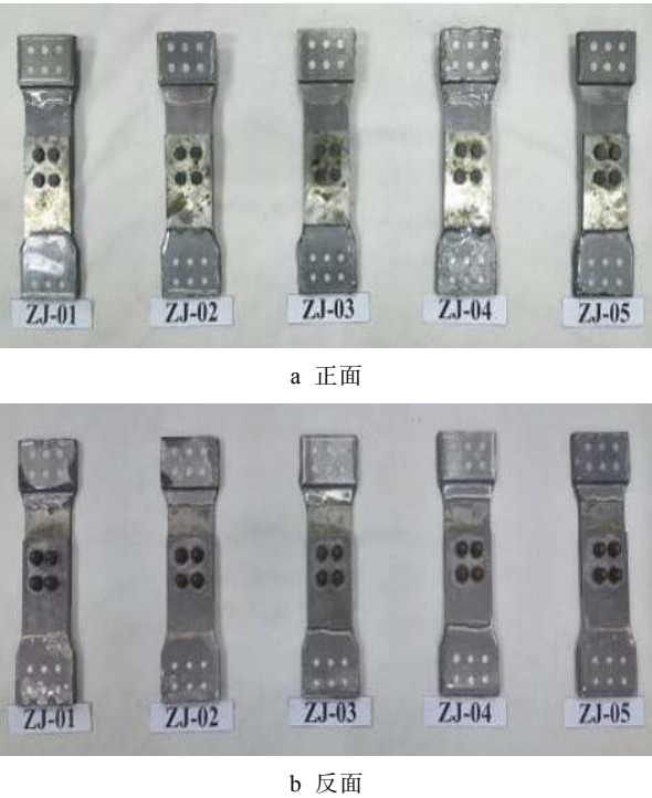
图 5 第 3 周期钢-钛搭接件宏观腐蚀形貌图 Fig.5 Macroscopic corrosion morphology of steel-titanium lap joints in the third cycle: a) front, b) back
