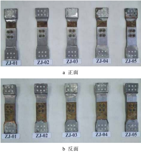
图 7 第 7 周期钢-钛搭接件宏观腐蚀形貌图 Fig.7 Macroscopic corrosion morphology of steel-titanium lap joints in the seventh cycle: a) front, b) back
