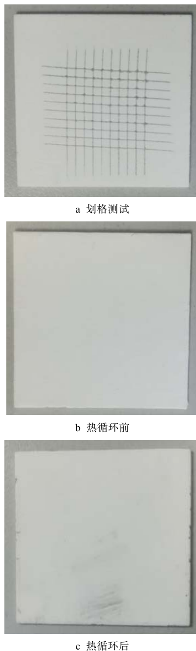
图7 涂层结合力测试 Fig.7 Bonding test of \text{Zn}_2\text{TiO}_4 inorganic thermal control coating: (a) cross cut test, (b) before thermal cycle, (c) after thermal cycle
