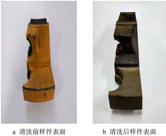
图 7 最优参数清洗前后的工件 Fig.7 Specimens before and after cleaning under optimal parameters: (a) before cleaning, (b) after cleaning
