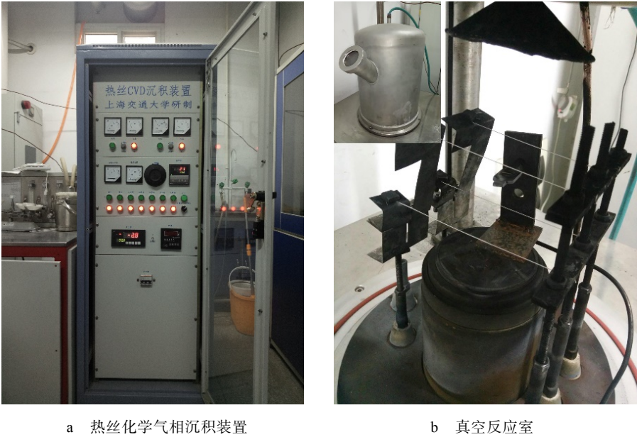
图 1 热丝化学气相沉积装置及真空反应室 Fig.1 Hot filament chemical vapor deposition (HFCVD) apparatus (a) and vacuum reaction chamber (b)
