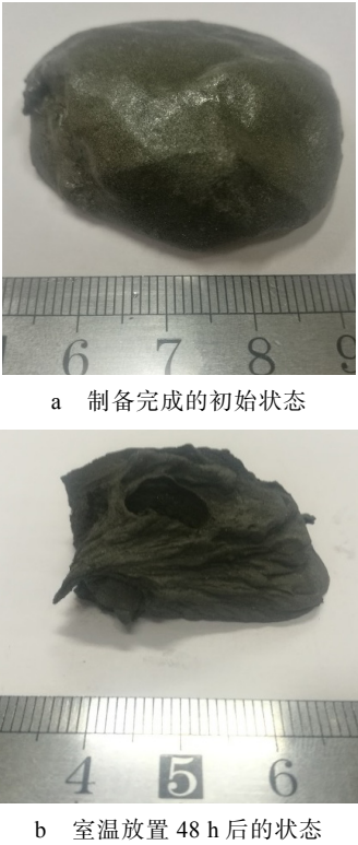
图 3 以 PVA 为基体制备的粘弹性磁性磨具室温固化 Fig.3 Room temperature curing of viscoelastic magnetic abrasive tool based on PVA: (a) initial state when preparation ends, (b) state after being placed at room temperature for 48 h
