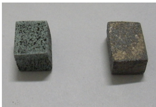
图 5 腐蚀溶液添加氟化铵前后镁合金的表观 Fig.5 Appearance of magnesium alloy before and after adding \text{NH}_4\text{F} to corrosion solution
