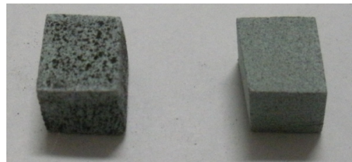
图 2 腐蚀溶液添加六次甲基四胺前后镁合金的表现 Fig.2 Appearance of magnesium alloy before and after adding hexamethylenetetramine to corrosion solution
