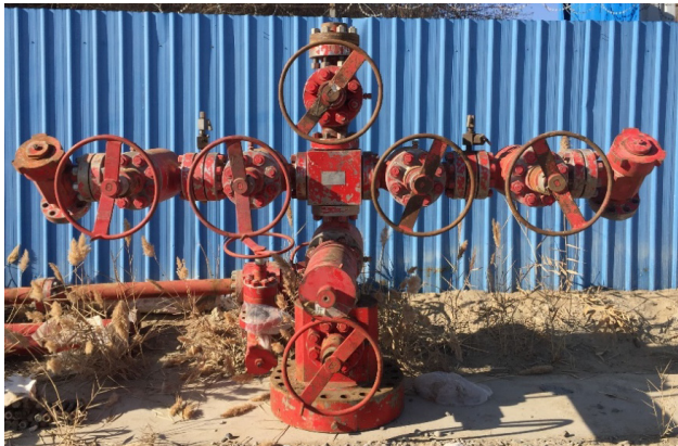
图 8 应急试采所用采气树实物 Fig.8 Gas production tree in kind for emergent trial production
