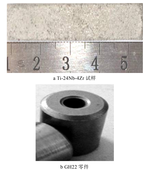
图 1 粉末冶金材料试样与粉末冶金零件 Fig.1 Powder metallurgy material sample and powder metallurgy parts: a) Ti-24Nb-4Zr sample; b) GH22 parts
