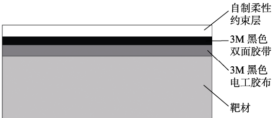
图 3 自制柔性约束层示意 Fig.3 The diagram of self-developed flexible confining medium
