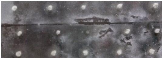
图 5 激光喷丸后的柔性约束层表面 Fig.5 Surface of flexible confining medium after laser peening
