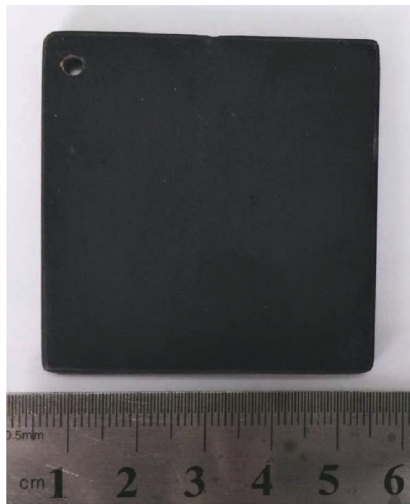
图 5 经过热循环测试 100 次后样品宏观照片 Fig.5 The appearance of the specimen after thermal cycle test of 100 times
