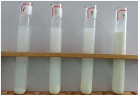
图 8 CeO 2 抛光液沉降实验结果 (CTAB 0.25 g/L SDBS 0.25 g/L PVP 15 g/L) Fig.8 Sedimentation experiment figure of CeO 2 polishing liquid (CTAB 0.25 g/L SDBS 0.25 g/L PVP 15 g/L)
