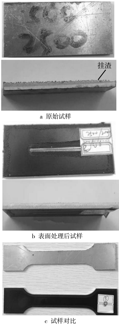
图 8 切割试样切缝及挂渣对比 Fig.8 Comparison of cutting specimen
