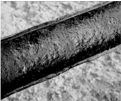
图 1 油管内壁宏观腐蚀形貌 Fig.1 Macro corrosion morphology of tubing inner wall
