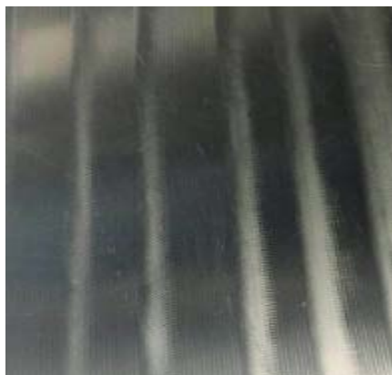
图 4 金刚石涂层立铣刀加工出来的表面 Fig.4 Surface processed by diamond coating end mill
