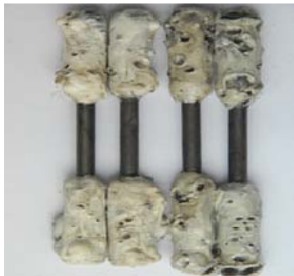
图 1 无预应力拉伸试样腐蚀后的宏观形貌 Fig.1 Macro-morphology of tensile samples without prestress after corrosion
