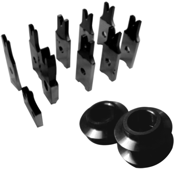
图 1 镀有类金刚石薄膜的模具 Fig. 1 Molds coated by diamond-like films
